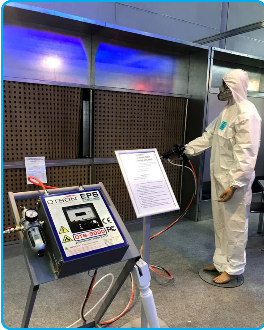
Dry Spray Booth
