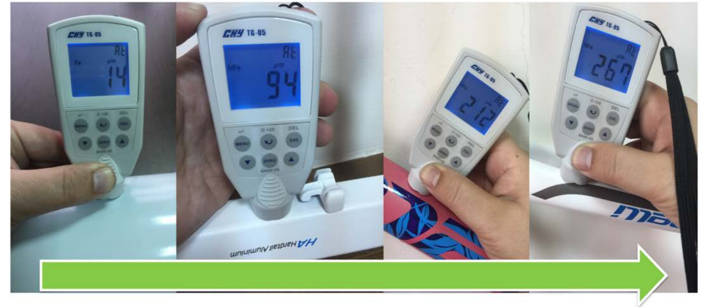
Different coatings thicknesses by OTSON Electrostatic Spray System
