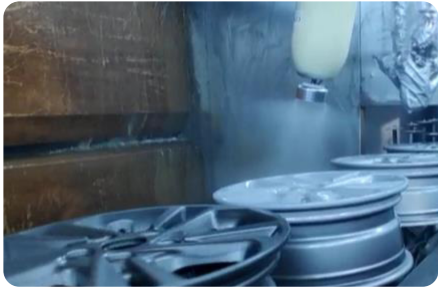
OTS - 7900 Auto Liquid Electrostatic Spray Bell
