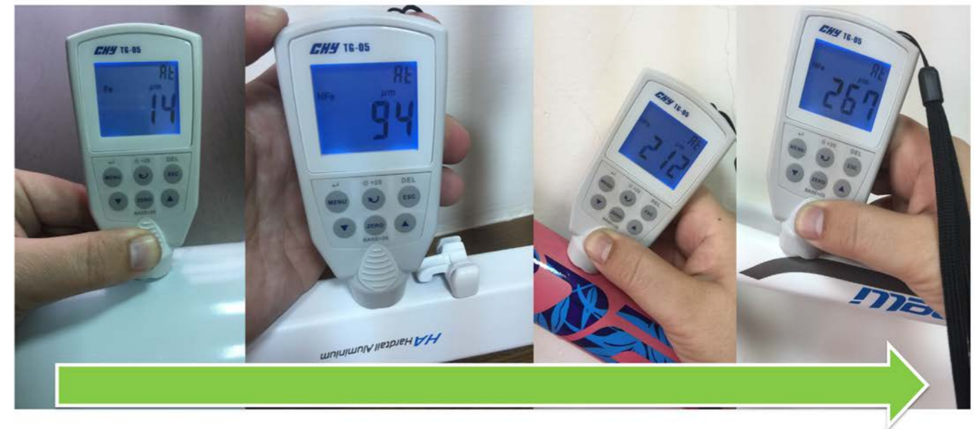
Different coatings thicknesses by OTSON Electrostatic Spray System
